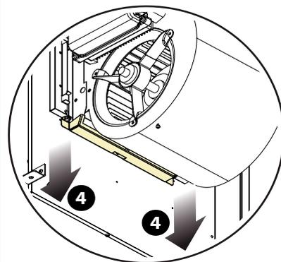
*Remove the two screws and bracket, highlighted (4), holding the fan housing, then lift slightly and remove it from the machine.*
